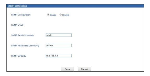
Main elements configuration description of SNMP configuration interface:
