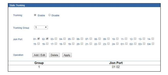
Step 5 Check the box of Port 1 and Port 2 in the "join port" bar.
