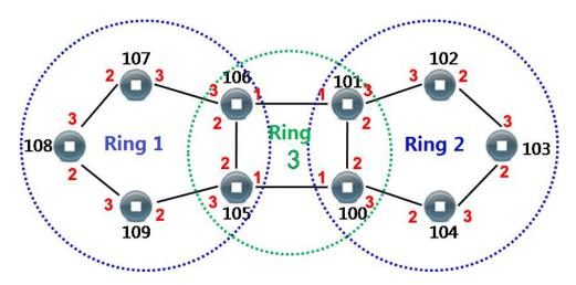
There are three rings in coupling ring. Ring 1 and Ring 2 intersect Ring 3 respectively. When setting ring in WEB interface, we can set Ring 1 and Ring 2 as single ring, Ring 3 as coupling ring. In coupling ring, we set the port in the link where the two rings intersect as control port. The Port 2 of Device 105 in the picture above is the control port. The analyses of each switch are displayed as follows:
