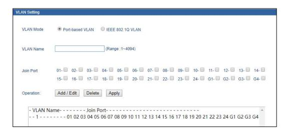
The main elements configuration description of port-based VLAN interface:
