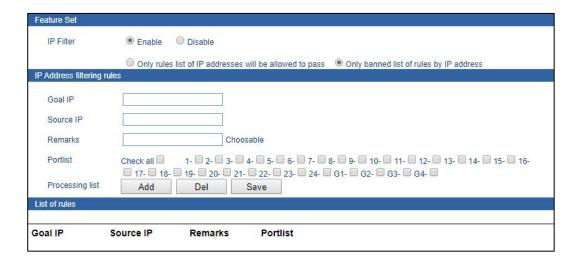
Main element configuration instructions in IP Filtering interface
