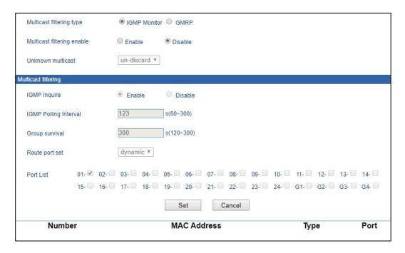
The main element configuration description of IGMP Snooping interface:
