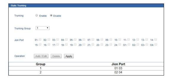
The main element configuration description of static trunking interface:
