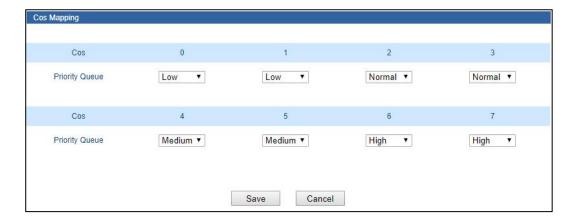
The main element configuration description of QoS mapping interface:
