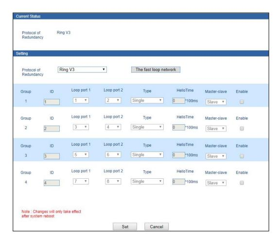
The main element configuration description of Ring network interface:
